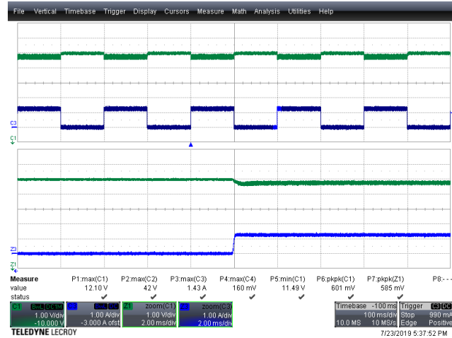
Figure 99 – Output Load Transient, 100% to 0% Load. V_{IN} = 60\text{ VDC} , I_{OUT} = 1.25\text{ A to }0\text{ A} . V_{OUT(MAX)} = 12.10\text{ V} , V_{OUT(MIN)} = 11.49\text{ V} . Upper: V_{OUT} , 1 V, 100 ms / div. Lower: I_{OUT} , 1 A, 100 ms / div. Bottom Half: Zoom @ 2 ms / div.
